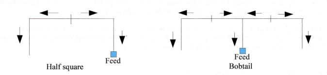
The Halfsquare works in a similar way to the two verticals shown earlier as a broadside array. Each vertical is approx a <sup>1</sup>/<sub>4</sub> wavelength and the horizontal top is <sup>1</sup>/<sub>2</sub> wavelength.
