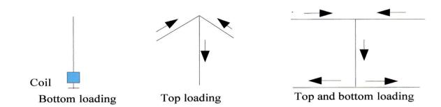
Bottom loading is the least efficient, keeping in mind the length of the wave and that the maximum current will be a ¼ wave from the far end of the antenna you can understand that most of the vertical will be high voltage and the max current will be in the coil.
