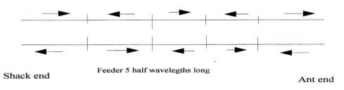
Notice how the currents are 180 degs out of phase with each other in each feedline, therefore providing the currents in the line are balanced there will be very little radiation from the line. Keeping the line away from metal objects usually is all that is needed to keep the line balanced.
