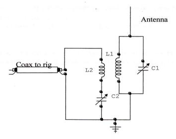
This simple Matching Unit can be made in a plastic lunchbox and placed right at the bottom of the vertical, fixed to a short wooden post if needed.
